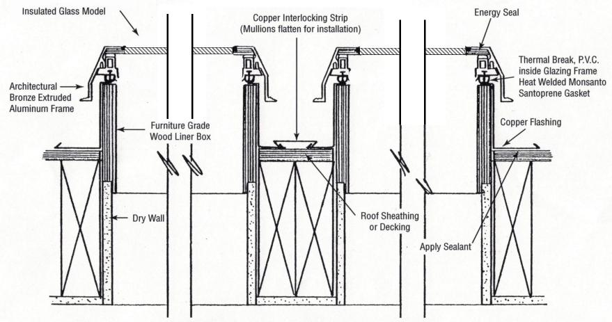
Installer Note: After installing skylights, Copper Interlock Strip has to be flattened flush to obtain proper seal. Use block of hard wood to close up copper until it is completely flattened. It is recommended that both interlock seams be soldered closed.
